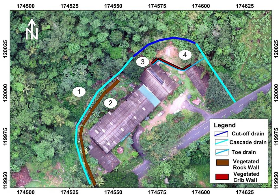
Fig. 3.1: Proposed drainage lay out
