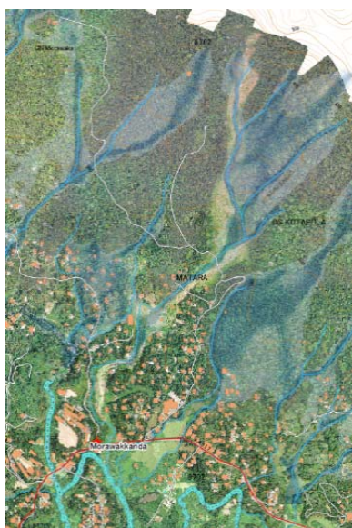
Figure 2.14: Hazard area validation in Morawakkanda Background image: drone image after debris flow Blue: simulated hazard probability of debris flow
